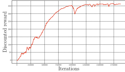
Fig. 4: Figure showing the discounted reward vs. the number of iterations. The reward saturates after approximately 1 million iterations.
